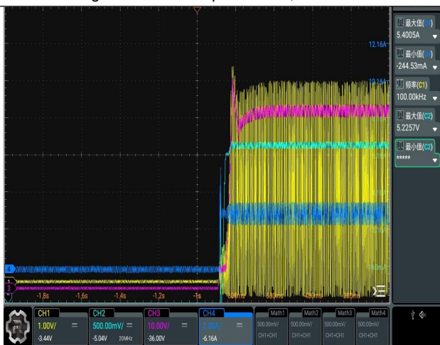
Ch1: SW Ch2: Vout Ch3: Vin Ch4: IL Vin=48V Vout=5V Fig.8-5 Vin Start up waveform, Iout =3A
