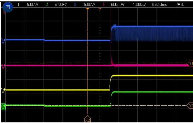
CH1: VIN CH2:VOUT CH3:SW CH4:IL Vin=5V Vout=5V Start up waveform through Vin, Iout =0A
