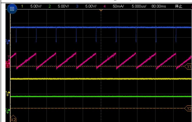
CH1: VIN CH2:VOUT CH3:SW CH4:IL Vin=5V Vout=5V Steady State waveform Iout =0A
