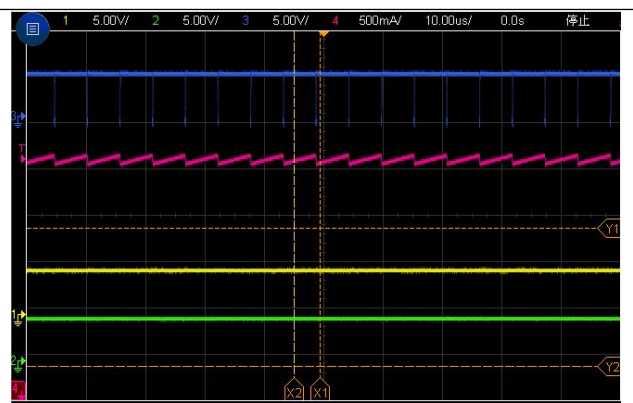
CH1: EN CH2:VOUT CH3:SW CH4:IL Vin=24V Vout=5V Shut Down waveform through EN, Iout =3A
