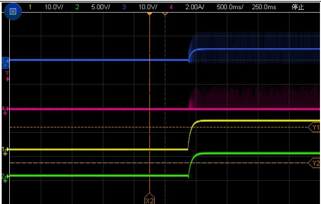
CH1: VIN CH2:VOUT CH3:SW CH4:IL Vin=5V Vout=5V Start up waveform through Vin, Iout =0A
