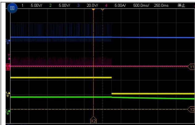
CH1: EN CH2:VOUT CH3:SW CH4:IL Vin=24V Vout=5V Shut Down waveform through EN, Iout =0A
