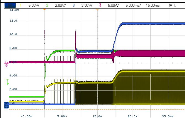
Fig.8-19 EN USM Start up waveform, Iout =2A
