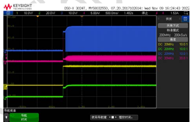
CH1: VIN CH2:VOUT CH3:SW CH4:IL Vin=16.8V Vout=20V Start up waveform through Vin, Iout =1A
