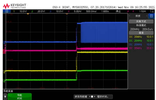
CH1: VIN CH2:VOUT CH3:SW CH4:IL Vin=20V Vout=20V Start up waveform through Vin, Iout =1A
