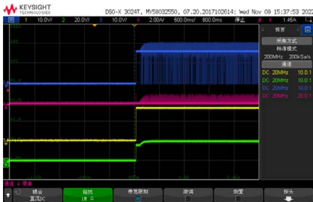
CH1: VIN CH2:VOUT CH3:SW CH4:IL Vin=16.8V Vout=20V Start up waveform through Vin, Iout =0A
