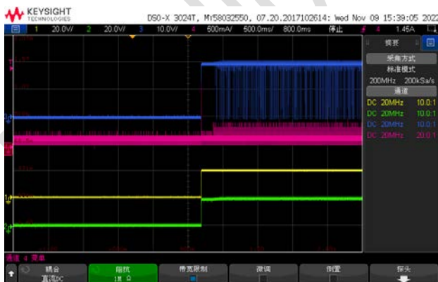
CH1: VIN CH2:VOUT CH3:SW CH4:IL Vin=20V Vout=20V Start up waveform through Vin, Iout =0A
